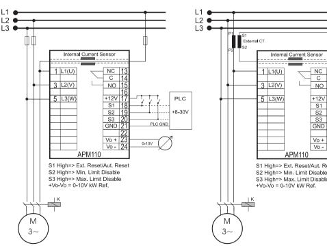
Fig.4 Typical connection with internal sensor
